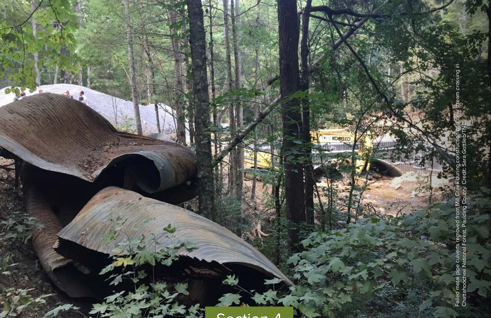
Failed metal pipe culverts removed from Mill Creek during construction of a new stream crossing in Chattahoochee National Forest, Paulding County. Credit: Sara Gottlieb/TNC
